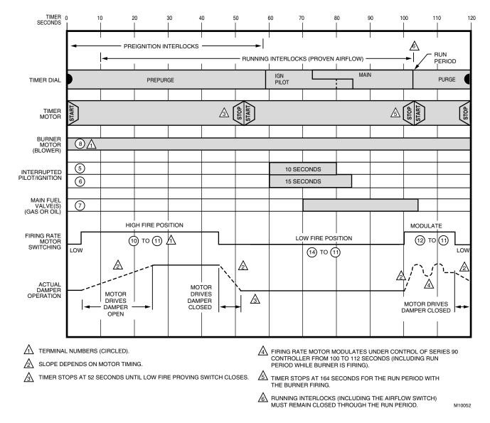
Fig. 6. Timer sequence for R4140G1106 Programmer.
